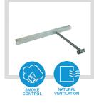
EA-K-50 24V DC 500N Chain Actuator Tested to EN12101-2 Available in: 300/500/600/ 750/1000/1200mm
