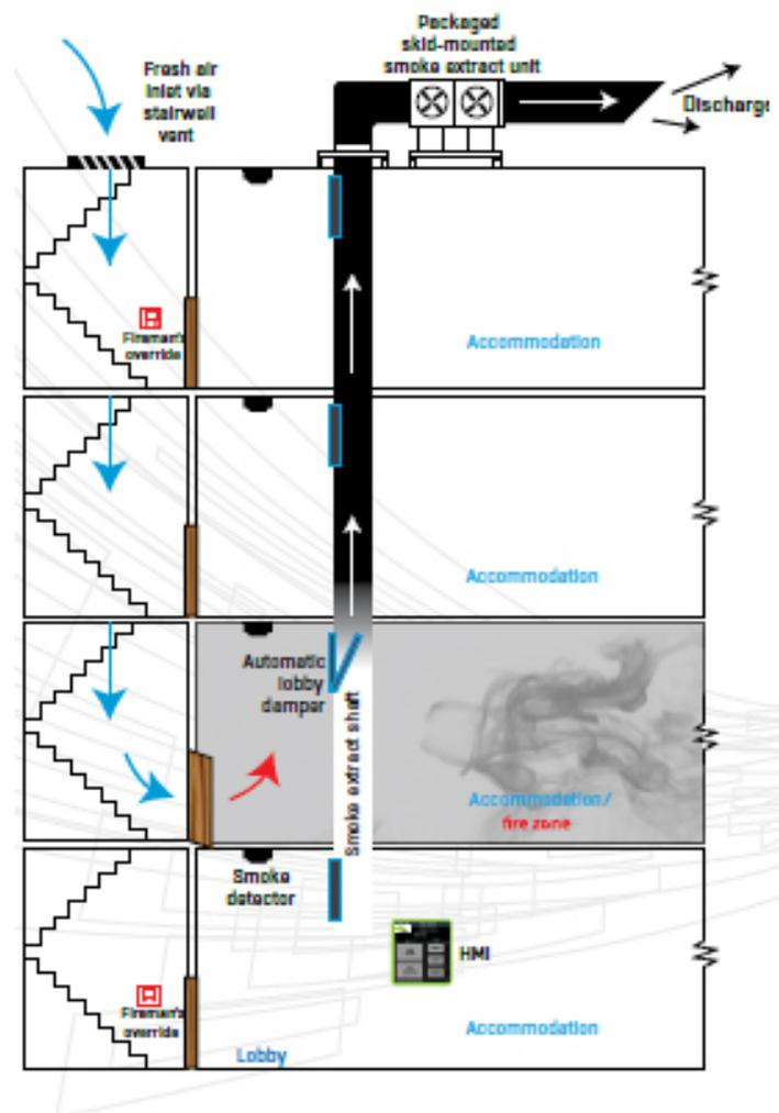
Figure 1 Mechanical smoke shaft illustration
